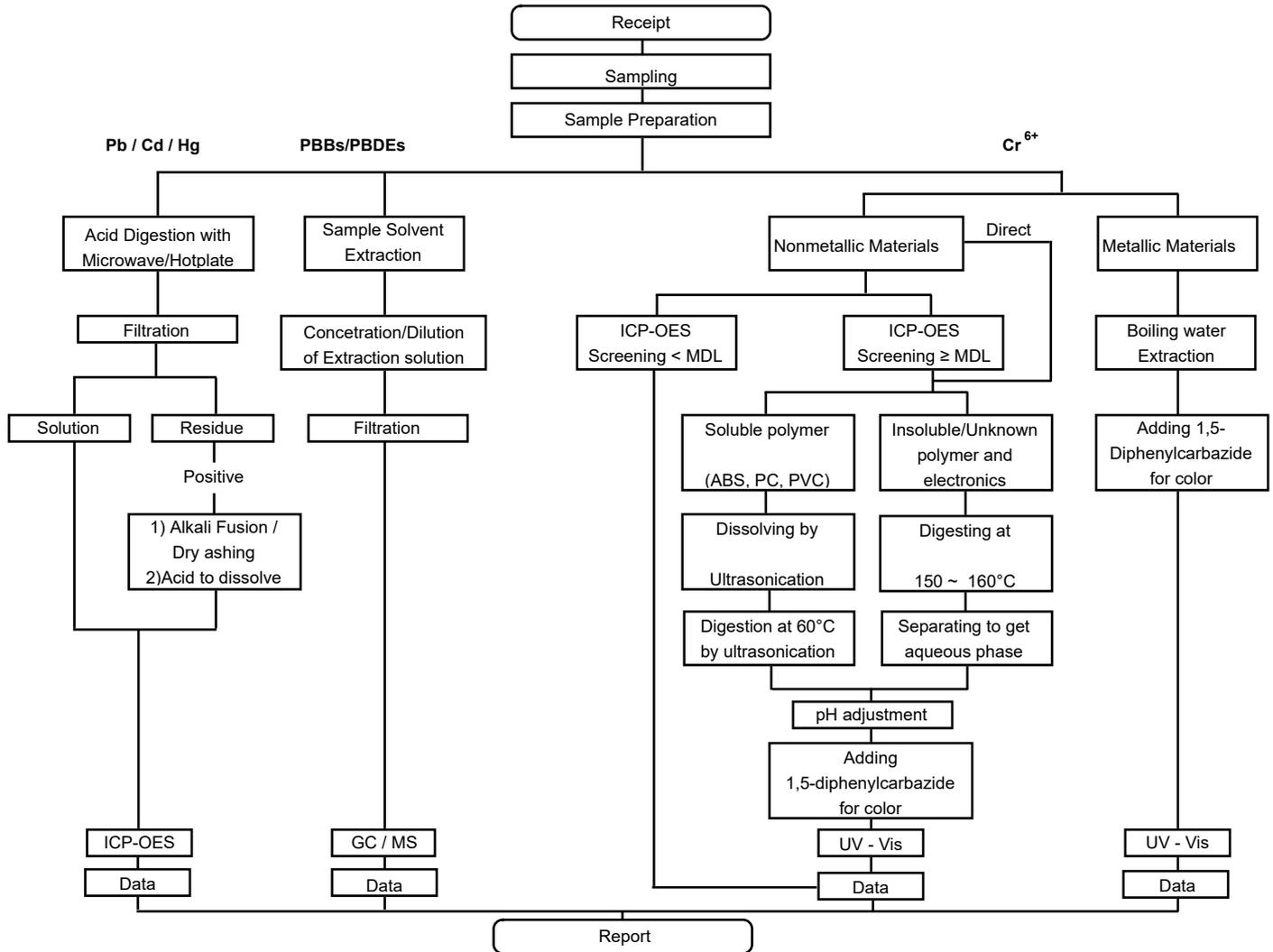
The samples were dissolved totally at the acid digestion step of the above flow chart for Cd, Pb, Hg.
